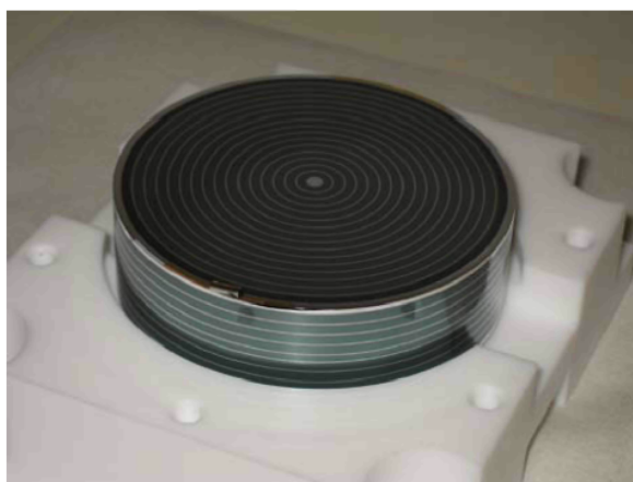
FIGURE 1. 400 g FID detector with its Ge-NTD sensor glued close to the edge of the absorber. Electrodes are connected between them by ultrasonic Aluminum bonding.
