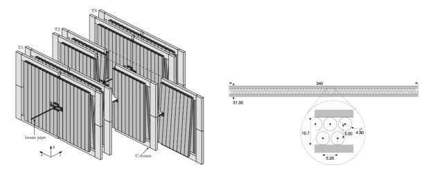
Figure 2.14 – a (Left) View of the OT. The T2 station is in open position. (Right) Illustration of the OT layer and zoom on the arrangement of straw tubes (distances are given in cm). [58]
