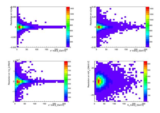
Figure 3.2 – Distributions versus  $p_z$  of  $\Delta_{\theta}$  (top, left),  $\Delta_{\phi}$  (top, right), and  $\Delta_{1/p_z}$  (bottom, left) for  $\pi^+$ , and distribution of  $\Delta_{m_{K^0_{\rm S}}}$  versus  $p_z$  (bottom, right).
