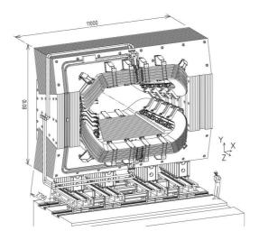
Figure 2.8 – Layout of the LHCb magnet.
