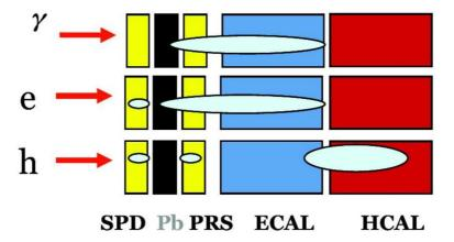
Figure 2.18 – Sketch of the typical repartition of showers depending on the nature of the incoming particle. "Pb" refers to a lead plate that converts photons to cascades of charged particles.
