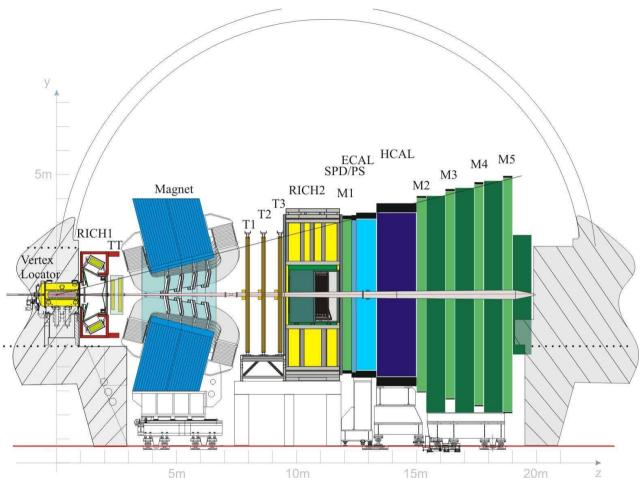
Figure 2.5 – Overview of the LHCb detector. The z axis is along the horizontal, while the y axis is along the vertical. The interaction point is located on the left, inside of the VELO subdetector. The beam pipe and the contours of the pit are filled with gray. Upstream and downstream directions correspond to the left and the right, respectively.
