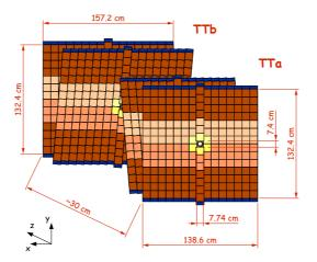
Figure 2.12 – Sketch of the TT subdetector. The two inner layers are tilted by a stereo angle of  $\pm 5^{\circ}$  (u/v-layers) in order to provide information on the y coordinate.
