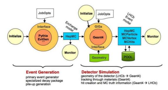
Figure 2.22 – The LHCb data processing applications and data flow. Underlying all of the applications is the Gaudi framework and the event model describes the data expected. The arrows represent input/output data
