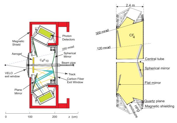
Figure 2.17 – Schematic cross section of the RICH1 (left) and RICH2 (right) detectors. [60]
