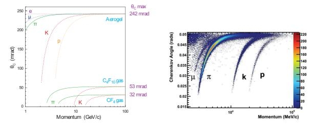
Figure 2.16 – (Left) Cherenkov angle as a function of the particle momentum for different radiators and particles. (Right) Reconstructed Cherenkov angle for isolated tracks, as a function of track momentum in the  $C_4F_{10}$  radiator [59]. The Cherenkov bands for muons, pions, kaons and protons are clearly visible.
