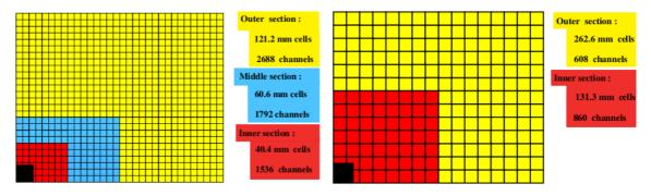
Figure 2.19 – (Left) Segmentation of the ECAL. (Right) Segmentation of the HCAL. The beam pipe region is filled with black, and is outside of the acceptance of both calorimeters.
