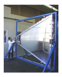
Figure 36: One MDC-IV in construction at IPN Orsay
