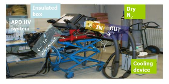
Figure 86: Set-up for the test of the PROTO60 prototype with cosmics at IPNO
