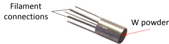
Figure 103: Anode used for alkali ion production
