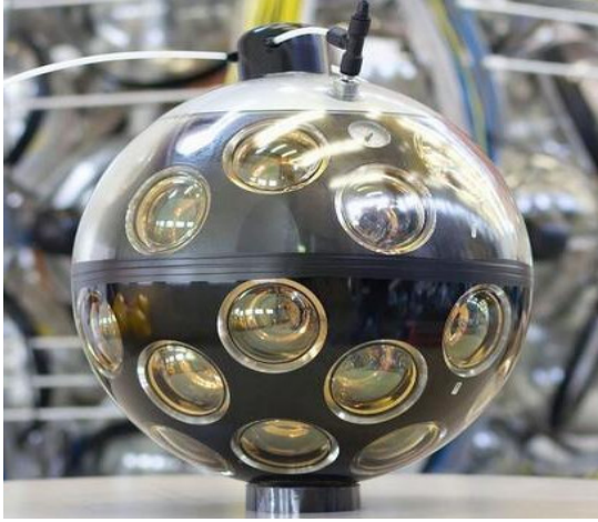
Figure 2.7: A photograph of a completed DOM.
