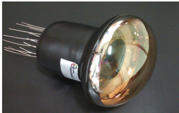
Figure 2.13: A photograph of a photomultiplier tube.
