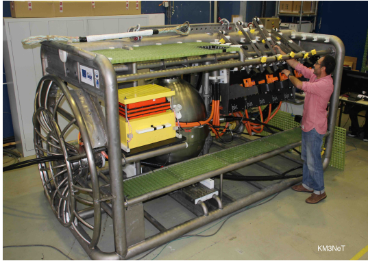
Figure 2.15: The first KM3NeT/ORCA junction box, photographed at CPPM before deployment.
