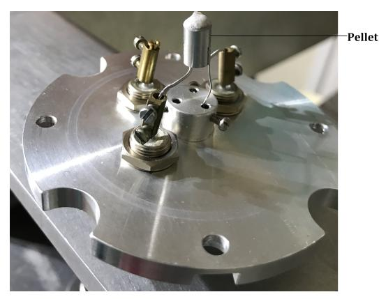
FIGURE 2.7: Actual setup with a sodium pellet connected to the two terminals.
